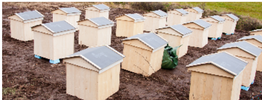
Small wooden houses used for testing PLEOT under natural climate conditions. Photo: Andreas Treu
