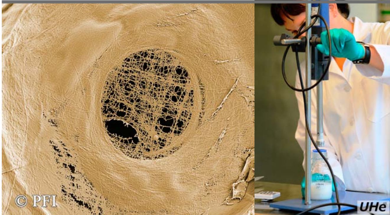
A magnified wood fibre from spruce, showing the cellulose nanofibrils and also a pore, covered by the fibrils (left), and emulsion preparation (right). Photo: Per Olav Johnsen, PFI (left) and Pia-Leena Heikkilä, University of Helsinki (right).
