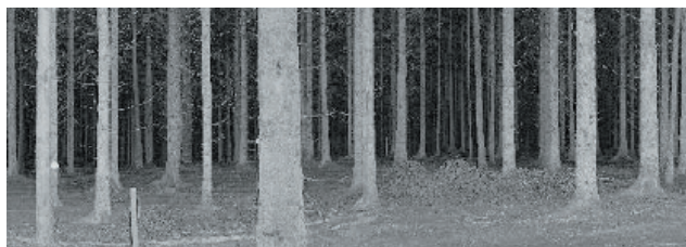
An intensity image produced by using the tree dimensional coordinates of reflection locations of laser pulses.
